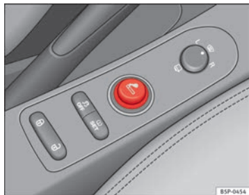
Fig. 116 The cigarette lighter is located in the power socket on the front of the centre console
