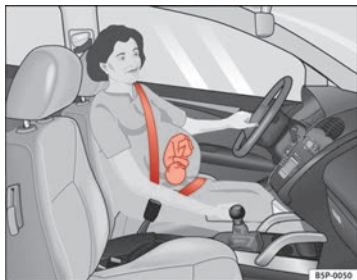
Fig. 15 Positioning seat belts during pregnancy
