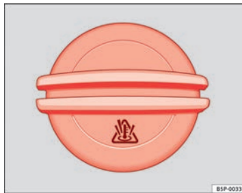
Fig. 168 In the engine compartment: Coolant expansion tank cap
