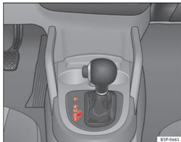
Fig. 146 Centre console: Selector lever for automatic gearbox / DSG automatic gearbox
