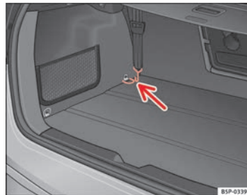
Fig. 128 Fastening rings for the separation net ▶
