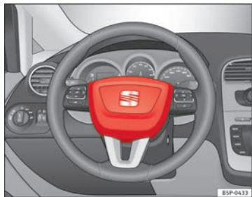
Fig. 18 Driver airbag located in steering wheel
