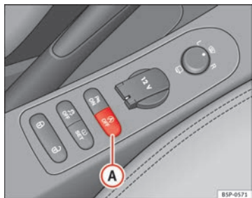
Fig. 142 The Start-Stop function button.
