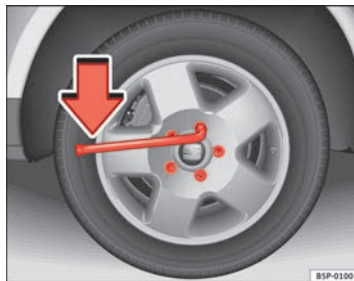
Fig. 180 Changing a wheel: loosen the wheel bolts
