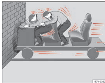
Fig. 8 The vehicle hits the wall: the occupants are not wearing seat belts
