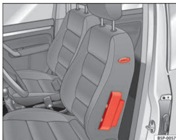
Fig. 22 Side airbag in driver seat
