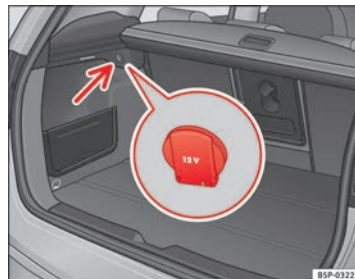
Fig. 118 Altea XL/Free-track Model: power socket in luggage compartment
