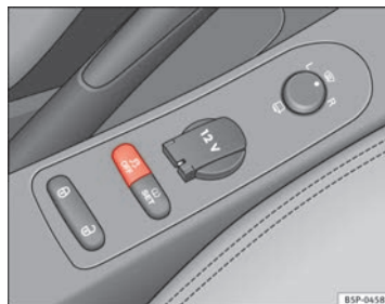
Fig. 139 Detailed view of the centre console: ESC switch.
