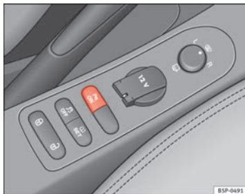
Fig. 153 Centre console: Switch for parking aid
