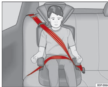
Fig. 30 Forward-facing child seat installed on rear seat
