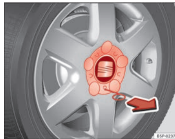
Fig. 179 Changing a wheel: Removing a hub cap
