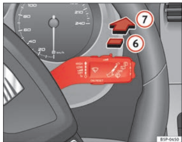
Fig. 86 Windscreen wiper and windscreen wash lever: rear window wiper
