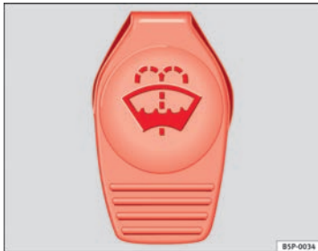
Fig. 169 In the engine compartment: Cap of windscreen washer fluid reservoir
