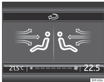
Fig. 134 Navigation display with information about the Climatronic
