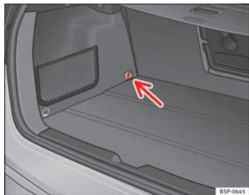
Fig. 32 Top Tether* securing ring
