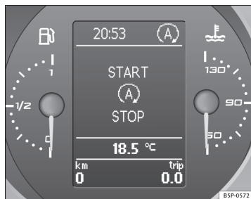
Fig. 143 Display on the instrument panel during Start-Stop function operation.
