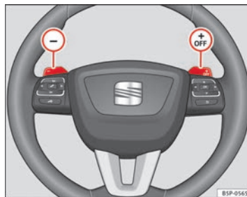
Fig. 151 Steering wheel with levers for automatic gearbox
