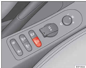
Fig. 141 Centre console: gas system control switch.
