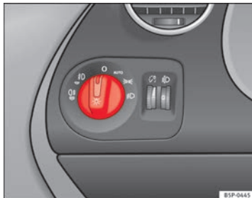
Fig. 72 Detailed view of the dash panel: lights, fog lights and rear fog light switch
