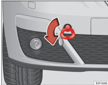
Fig. 203 The front right section of the vehicle: Fitting the front towline anchorage
