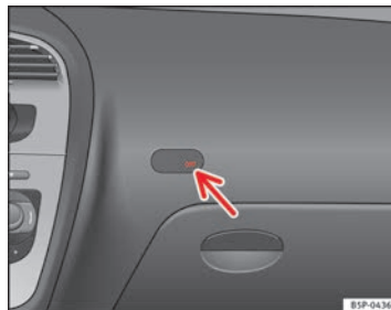
Fig. 27 Control lamp for deactivated front passenger airbag in centre console
