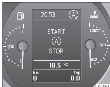
Fig. 138 Display on the instrument panel during Start-Stop function operation.
