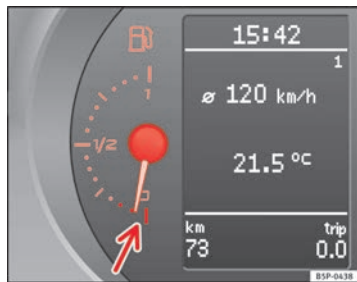
Fig.35 Instrument panel: fuel gauge
