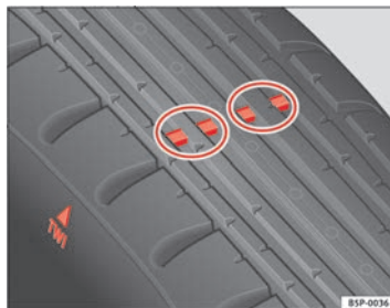
Fig. 172 Tyre tread wear indicators
