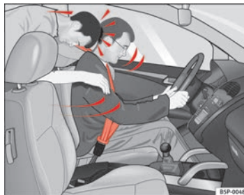
Fig. 10 The unbelted rear passenger is thrown forward violently, hitting the driver wearing a seat belt.
