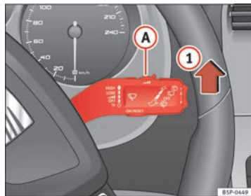
Fig. 87 Windscreen wiper lever
