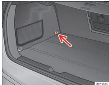
Fig. 32 Top Tether* securing ring
