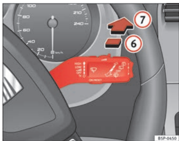
Fig. 88 Windscreen wiper and windscreen wash lever: rear window wiper
