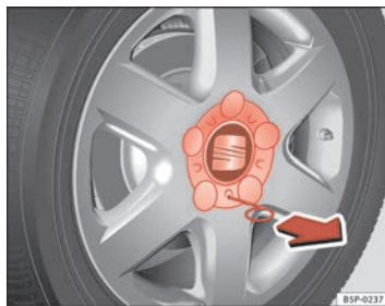
Fig. 175 Changing the wheel: Removing a hub cap
