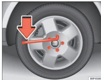
Fig. 176 Changing the wheel: loosen the wheel bolts
