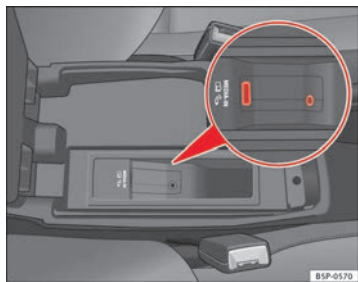
Fig. 121 Connection in central armrest compartment
