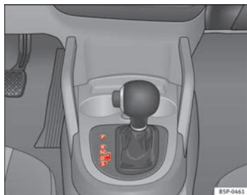
Fig. 142 Centre console: Selector lever for automatic gearbox / DSG automatic gearbox
