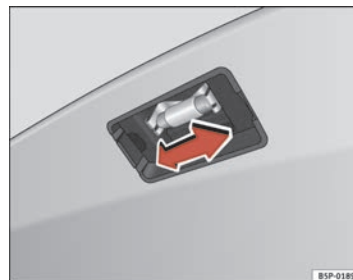
Fig. 200 Number plate light
