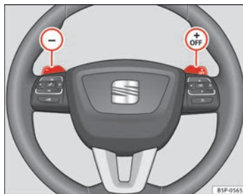
Fig. 147 Steering wheel with levers for automatic gearbox
