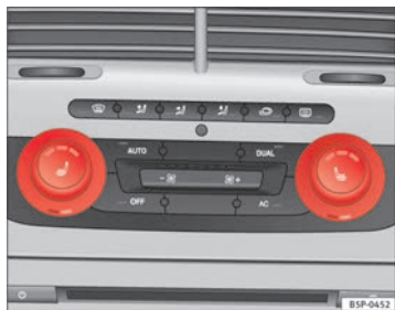
Fig. 96 Front seat heating with Climatronic
