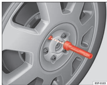
Fig. 179 Changing the wheel: Hexagonal socket in screwdriver handle to turn the wheel bolts
