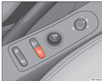
Fig. 52 Centre console: tyre monitor system button
