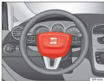
Fig. 18 Driver airbag located in steering wheel
