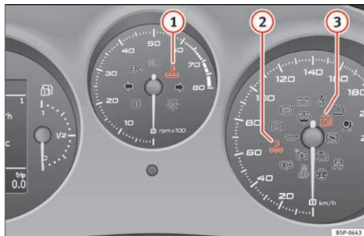
Fig. 51 Instrument panel indicator and warning lamps in vehicles with LPG.
