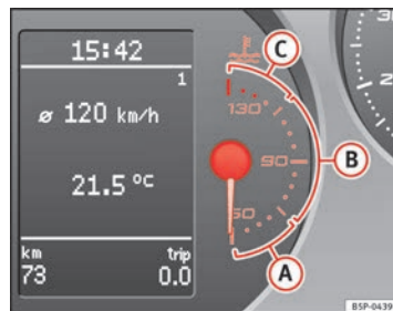
Fig.36 Instrument panel: engine coolant temperature gauge
