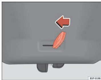
Fig. 68 Tailgate: emergency open
