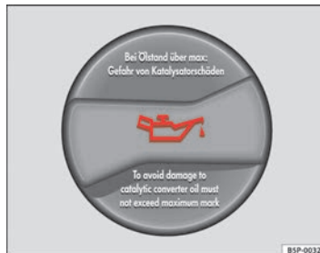
Fig. 164 In the engine compartment: Engine oil filler cap
