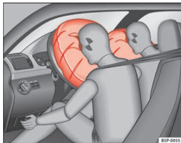
Fig. 20 Inflated front airbags
