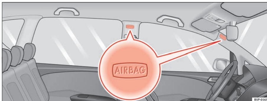
Fig. 24 Location of left curtain airbag
