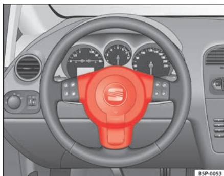
Fig. 18 Driver airbag located in steering wheel
