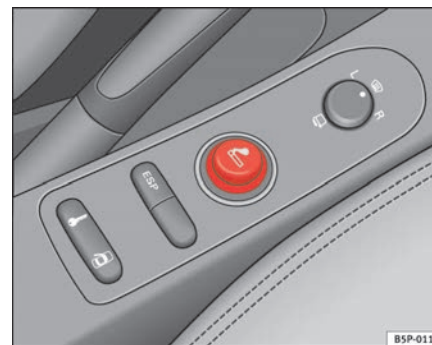
Fig. 116 The cigarette lighter is located in the electric socket on the front of the centre console
