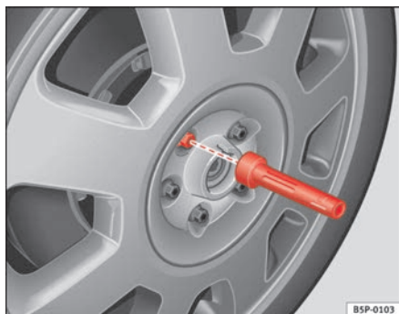
Fig. 178 Changing the wheel: hexagonal socket in screwdriver handle to turn the wheel bolts after they have been loosened
