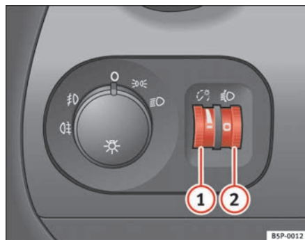
Fig. 75 Instrument panel: regulation for instrument and switch illumination and headlight range control
