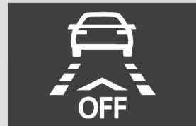
Fig. 250 On the instrument panel display: Front Assist deactivated indication.
