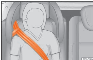
Fig. 35 Integrated child seat: seat belt route with guide handle.
