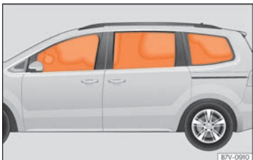
Fig. 25 Deployed head-protection airbags.
