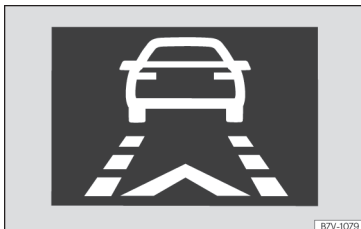
Fig. 249 On the instrument panel display: advance warning indications.
