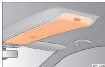
Fig. 159 On the roof console: storage compartment.
