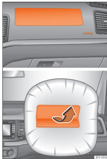
Fig. 17 Front passenger airbag located in dash panel.
