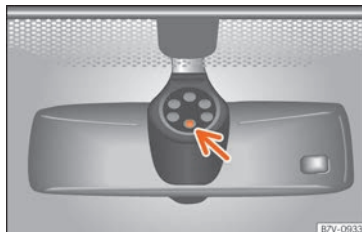
Fig. 122 Rain sensor sensitive surface
