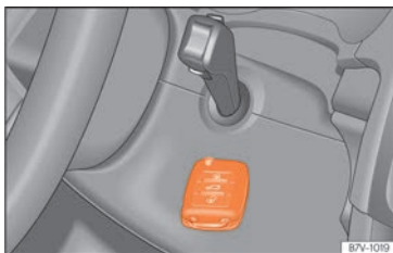
Fig. 232 Emergency ignition in vehicles with Keyless Access.
