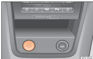
Fig. 231 In the centre console: Start button of the Keyless Access locking and starting system. The layout in right-hand drive vehicles is symmetrical.
