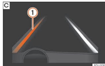
Fig. 258 On the instrument panel display: Indication on the Lane Assist system display (example 2).
