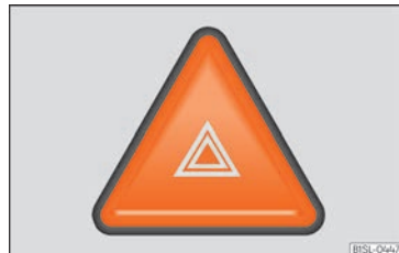
Fig. 117 Dash panel: hazard warning lights switch
