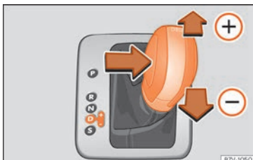
Fig. 236 Selector lever in Tiptronic position (left-hand drive vehicles). The lay-out in right-hand drive vehicles is symmetrically opposed.
