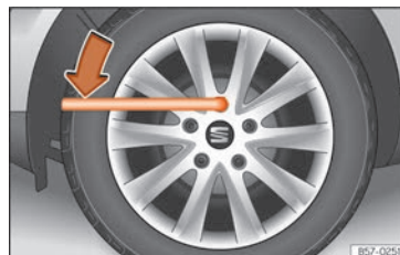
Fig. 45 Wheel change: loosen the wheel nuts.
