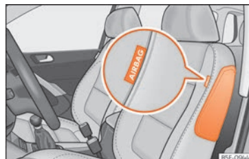
Fig. 22 Side airbag in driver's seat.
