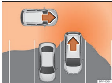
Fig. 262 Schematic representation of the rear cross traffic alert assistant: zone monitored around the vehicle while leaving a parking space.
