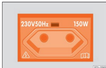
Fig. 172 Detailed view of the rear centre console: 230 volt European power socket.
