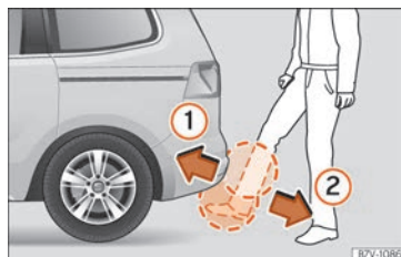
Fig. 106 Rear lid with sensor-controlled opening (Easy Open).
