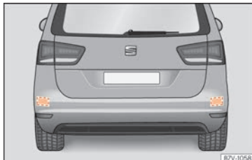
Fig. 244 Rear view of the vehicle: radar sensor zones.
