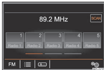
Fig. 200 Radio mode: automatic playback (SCAN) active.
