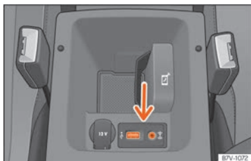
Fig. 231 Centre front armrest: USB/AUX-IN input.
