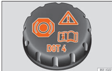
Fig. 292 Engine compartment: brake fluid reservoir cap.
