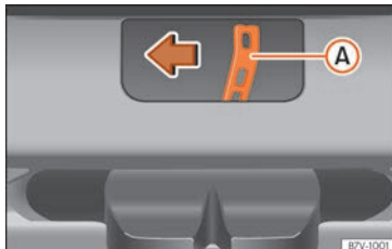
Fig. 108 Detail of the luggage compartment: emergency unlocking
