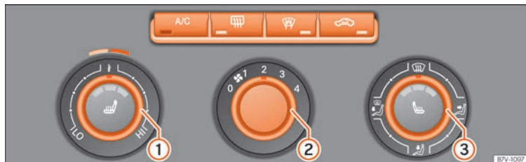
Fig. 174 In the centre console: manual air conditioning controls.
