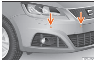
Fig. 272 Parking sensor system sensors on the front bumper
