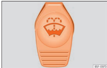
Fig. 293 In the engine compartment: blue cap of the windscreen washer tank.
