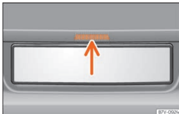
Fig. 105 Opening the boot hatch from the outside
