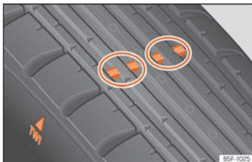
Fig. 296 Tyre profile: tread wear indicators.
