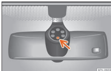
Fig. 122 Rain sensor sensitive surface
