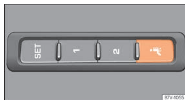
Fig. 135 On the side of the front seat: button for the lumbar massage function.
