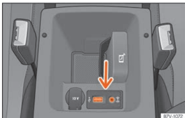
Fig. 185 Centre front armrest: USB/AUX-IN input.
