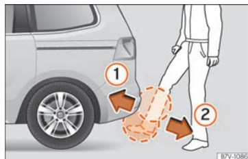
Fig. 106 Rear lid with sensor-controlled opening (Easy Open).
