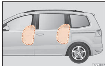
Fig. 23 Range of action of the front and rear side airbags. With 5 and 7 seats. »
