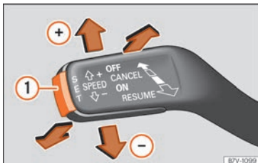
Fig. 251 On the left of the steering column: third lever for operating the GRA.
