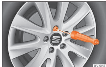
Fig. 49 Wheel change: loosen wheel nuts with the socket in the handle of the screwdriver.
