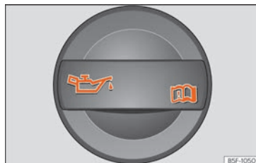
Fig. 289 In the engine compartment: Engine oil filler cap.
