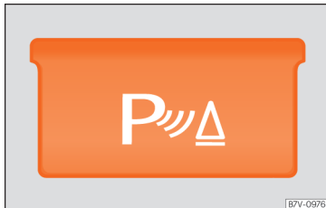
Fig. 271 Detailed view of the centre console: button to connect or disconnect the park assist.
