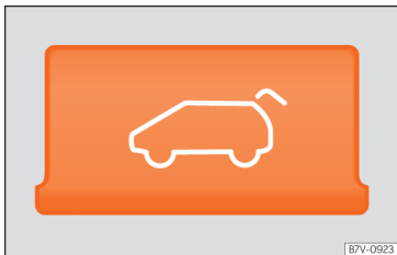
Fig. 102 Detailed view of the centre console: rear lid unlocking button.
