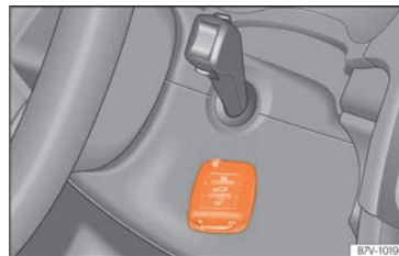
Fig. 235 Emergency ignition in vehicles with Keyless Access.
