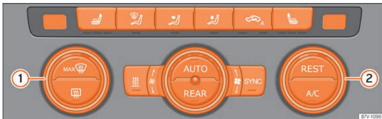
Fig. 173 In the centre console: Climatronic controls.
