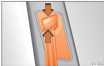
Fig. 15 Next to the front seats: belt height adjuster.
