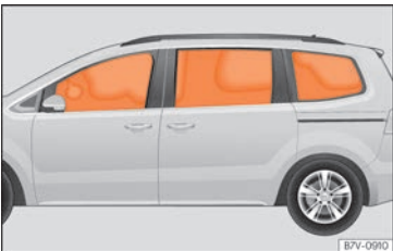
Fig. 25 Deployed head-protection airbags.
