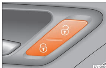
Fig. 90 Driver's door: central locking switch.
