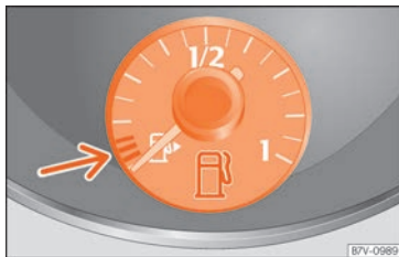
Fig. 78 On the instrument panel: fuel gauge.
