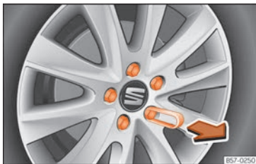
Fig. 43 Wheel: wheel nuts with caps.
