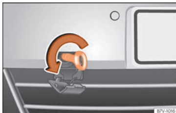
Fig. 56 On the right side of the front bumper: screw in the towline anchorage
