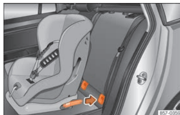
Fig. 30 Rear seats: fitting a child seat with the ISOFIX system.
