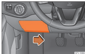
Fig. 58 On the driver's side dashboard: fuse box cover.
