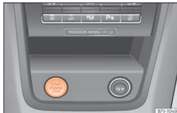
Fig. 234 In the centre console: Start button of the Keyless Access locking and starting system. The layout in right-hand drive vehicles is symmetrical. »
