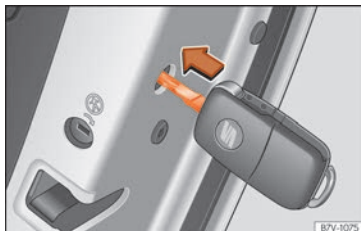
Fig. 97 Emergency locking of the vehicle using the vehicle key
