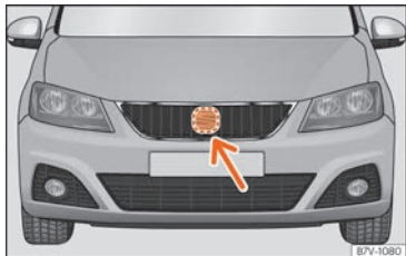
Fig. 244 On the front bumper: radar sensors.
