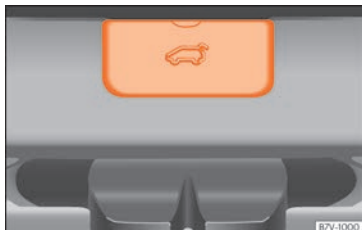
Fig. 107 Detail of the luggage compartment: access to emergency unlocking.
