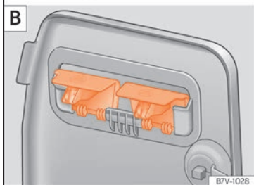
Fig. 142 Remove the shelf supports A then put them away safely B.
