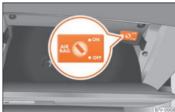
Fig. 18 In the glove compartment, on the front passenger side: key switch for activating and deactivating the front passenger airbag.
