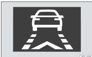
Fig. 252 On the instrument panel display: advance warning indications.
