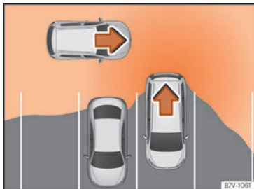
Fig. 265 Schematic representation of the rear cross traffic alert assistant: zone monitored around the vehicle while leaving a parking space.
