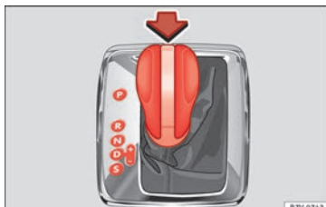
Fig. 130 Automatic gearbox selector lever with locking button (arrow)
