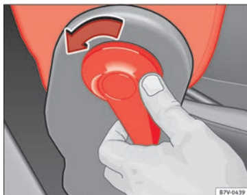
Fig. 85 Unlocking the folding seat backrest of the front passenger seat
