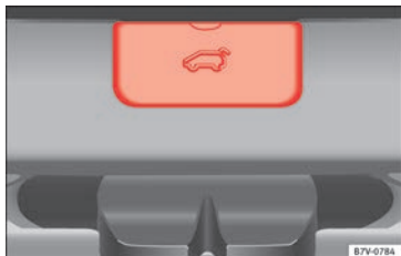
Fig. 199 From the luggage compartment: remove the boot hatch cover.
