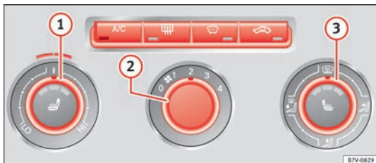
Fig. 120 Detailed view of the centre console: Electronic manual air conditioning controls
