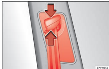
Fig. 12 Next to the front seats: belt height adjuster
