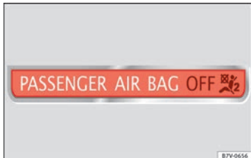
Fig. 21 Control lamp for disabling the front passenger front airbag on the dash panel
