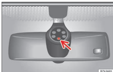
Fig. 68 Rain sensor sensitive surface
