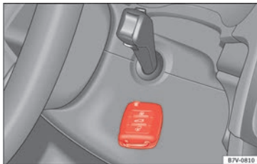
Fig. 127 Emergency ignition in vehicles with KESSY.
