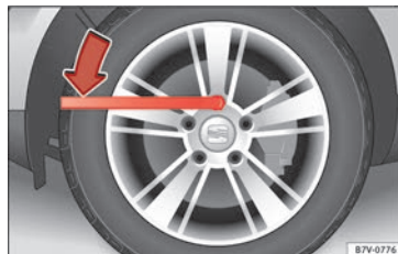
Fig. 185 Changing a wheel: Slacken the wheel bolts.
