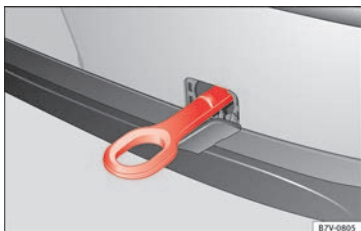
Fig. 195 On the rear bumper, to the right hand side: Tow ring in position
