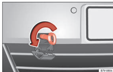
Fig. 194 On the right-hand side of the front bumper: Screw in the towline anchorage.
