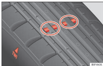
Fig. 176 Tyre tread: tread wear indicators
