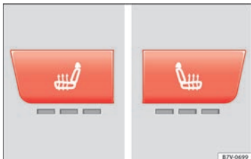
Fig. 81 Detailed view of the centre console: controls for the front seat heating in vehicles equipped with Climatronic
