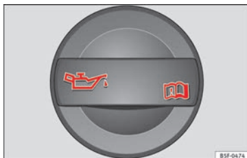
Fig. 166 In the engine compartment: Engine oil filler cap.
