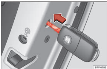
Fig. 198 Emergency locking of the vehicle using the vehicle key
