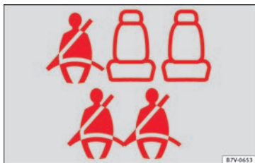
Fig. 5 Example of seat belt status display for the rear seats (here, a 7-seat vehicle) on the instrument panel above, the second row and, below, the third row of seats.
