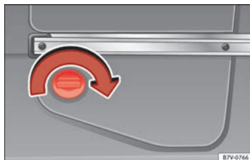
Fig. 160 At the rear left of the luggage compartment: AdBlue tank, behind a cover panel
