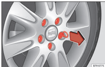
Fig. 184 Removing the wheel bolt caps
