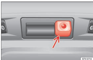
Fig. 143 On the rear lid: location of the rear assist camera
