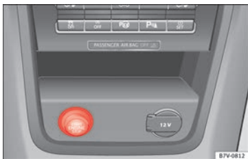
Fig. 126 In the centre console: start-up push button for the Keyless Access lock and start-up system. The layout in right-hand drive vehicles is symmetrical.
