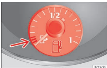
Fig. 158 On the instrument panel: Fuel gauge for petrol and diesel
