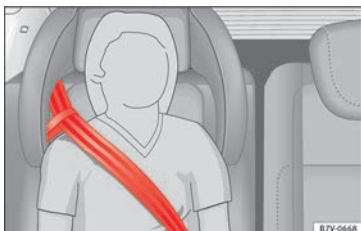
Fig. 31 Integrated child seats. seat belt routing with guide handle
