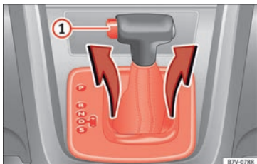
Fig. 203 Remove the lining from the area of the gear indication
