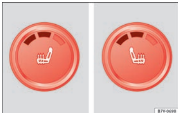
Fig. 80 Detailed view of the centre console: front seat heating controls, here with the second temperature level set
