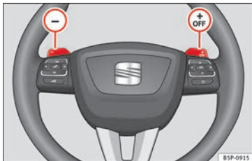
Fig. 132 Steering wheel with two paddle shifts for Tiptronic
