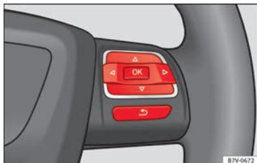
Fig. 37 Multifunction steering wheel: buttons to access the instrument panel menus
