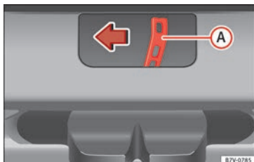
Fig. 200 From the luggage compartment: Emergency unlocking of the boot hatch.
