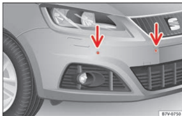
Fig. 138 Parking sensor system sensors on the front bumper
