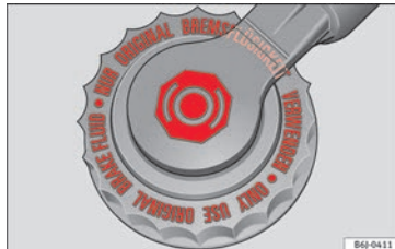
Fig. 170 In the engine compartment: brake fluid reservoir cap
