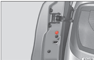
Fig. 197 To the front of the passenger side door: Emergency lock, hidden by a rubber cap.
