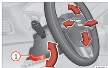
Fig. 3 Mechanical steering wheel adjustment
