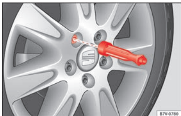
Fig. 189 Changing a wheel: loosen wheel bolts with the socket at the end of the wheel brace
