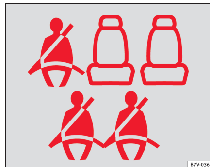
Fig. 4 Example of seat belt status display for the rear seats (here, a 7-seat vehicle) on the instrument panel, above the second row and below the third row of seats.
