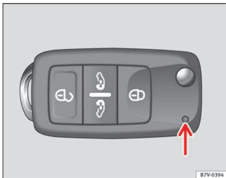
Fig. 42 Indicator light on the vehicle key for vehicles with electric sliding doors.
