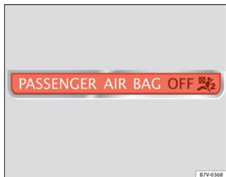
Fig. 16 Warning lamp for disabling the front passenger airbag on the instrument panel.
