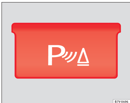
Fig. 140 Detailed view of the centre console: button for switching the parking sensor system on and off.
