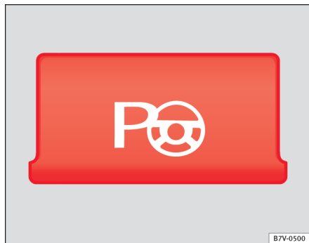
Fig. 144 Detailed view of the centre console: button to switch the park assist system on manually.
