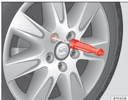
Fig. 185 Changing the wheel: loosen wheel bolts with the socket at the end of the wheel brace.
