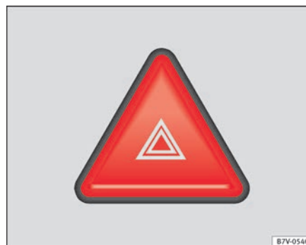
Fig. 186 In the centre of the instrument panel: Switch for hazard warning lights.
