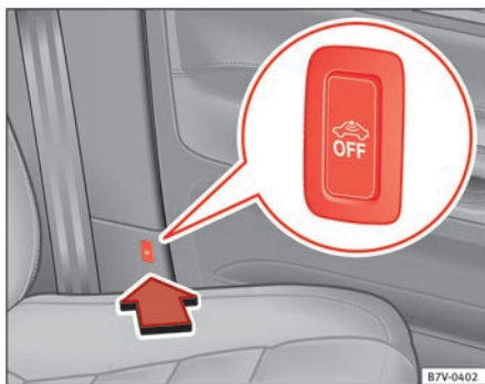
Fig. 48 Driver's seat: button for switching off the interior monitoring system and the anti-tow system.
