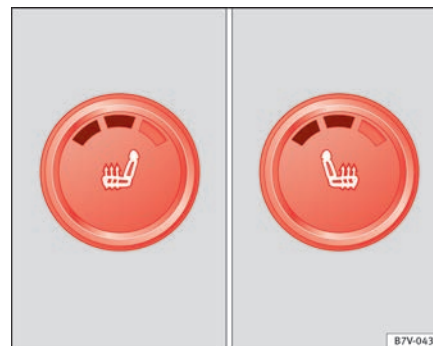
Fig. 79 Detailed view of the centre console: front seat heating controls, here with the second temperature level set.
