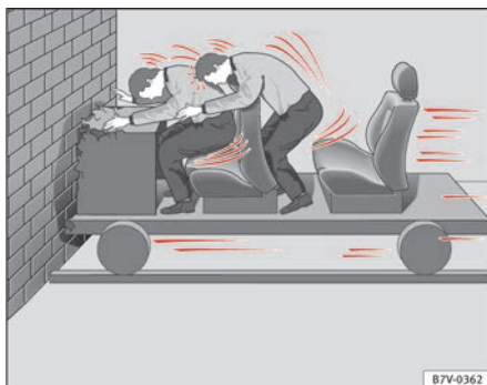
Fig. 6 The vehicle hits the wall: the occupants are not wearing seat belts.
