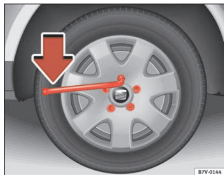
Fig. 158 Changing the wheel: loosen the wheel bolts
