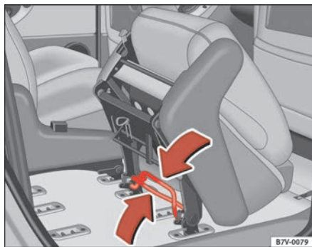
Fig. 92 Bar for removing and installing the individual seat
