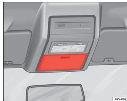
Fig. 103 Stowage area in the roof
