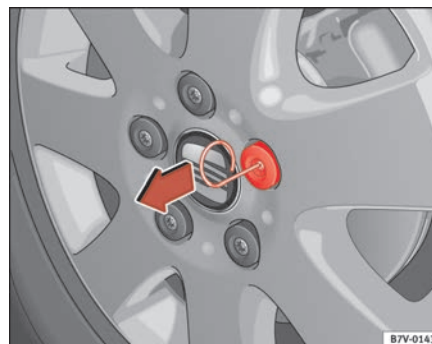
Fig. 157 Use the hook to pull off the cap
