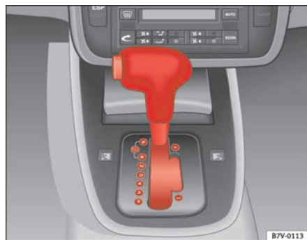
Fig. 130 Centre console: gearbox selector lever with locking button
