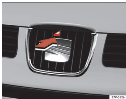
Fig. 139 Detail of radiator grille: lever for unlocking the bonnet.
