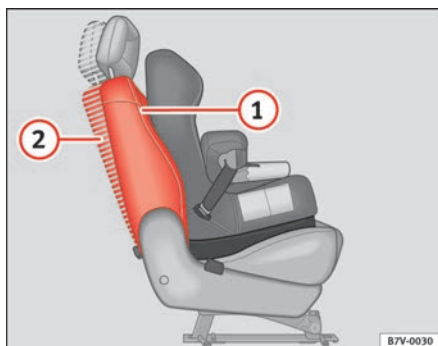
Fig. 34 Backrest adjustment when using ISOFIX child seats
