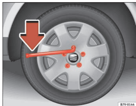
Fig. 158 Changing the wheel: loosen the wheel bolts
