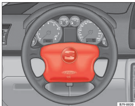
Fig. 22 Driver airbag located in steering wheel
