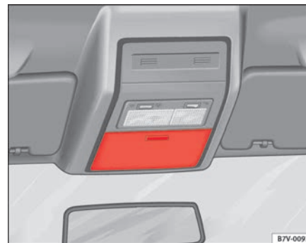
Fig. 103 Stowage area in the roof
