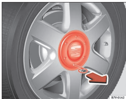
Fig. 156 Removing the hubcaps
