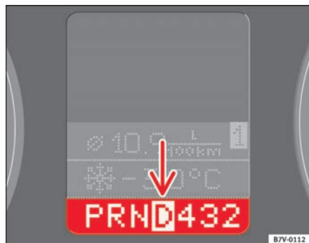
Fig. 131 Instrument panel: display showing position of selector lever
