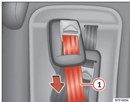
Fig. 38 Integrated child seats. adjusting harness belt
