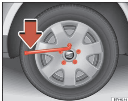
Fig. 157 Changing the wheel: loosen the wheel bolts
