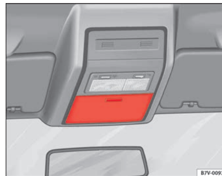
Fig. 103 Stowage area in the roof
