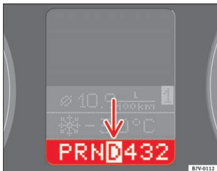
Fig. 130 Instrument panel: display showing position of selector lever
