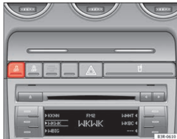
Fig. 152 Centre console with ESC switch
