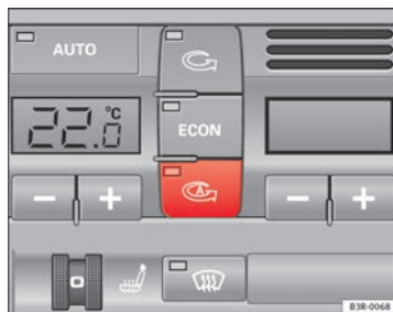
Fig. 129 Button for automatic air recirculation
