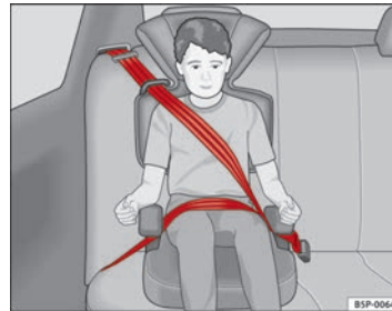
Fig. 31 Forward-facing child seat installed on rear seat.
