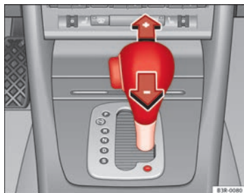
Fig. 149 Centre console: Manual gear selection (tiptronic mode)
