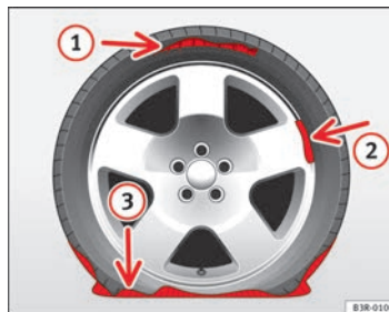
Fig. 186 The Tyre Mobility System is not suitable for repairing this type of damage to tyres.
