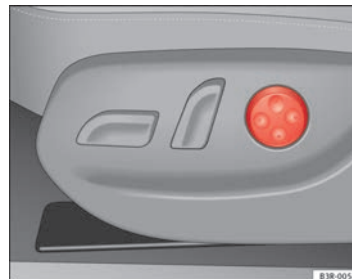
Fig. 107 Front seat: Adjuster switch for lumbar support
