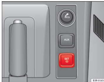
Fig. 176 Detailed view of the centre console: Button for the tyre pressure monitoring system
