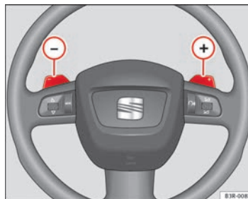
Fig. 151 Steering wheel: tiptronic controls
