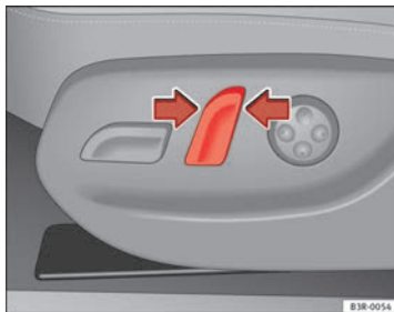
Fig. 106 Front seat: Backrest adjuster switch
