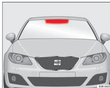
Fig. 165 Location of the electronic toll collection system
