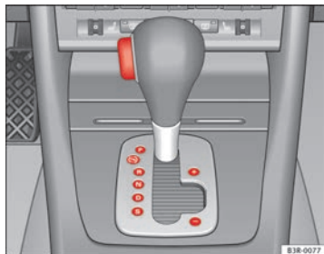
Fig. 146 Detailed view of the centre console: Selector lever with lock button
