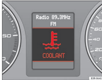
Fig. 54 Display: Coolant level warning
