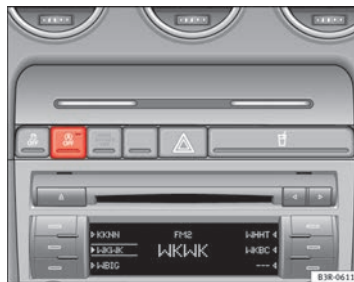
Fig. 136 The Start-Stop function button.
