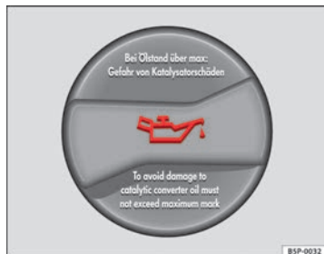
Fig. 170 In the engine compartment: Engine oil filler cap
