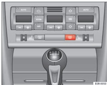
Fig. 95 Switch for heated rear window
