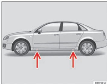
Fig. 183 Changing the wheel: Jack position points
