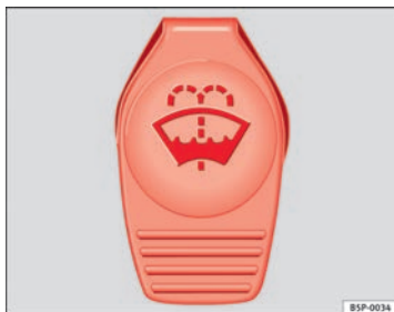
Fig. 172 In the engine compartment: Cap of windscreen washer fluid reservoir.
