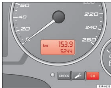
Fig. 42 Detailed view of the instrument panel: Odometer
