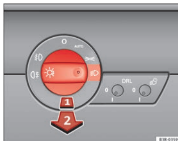
Fig. 82 Detailed view of the dash panel: Light switch
