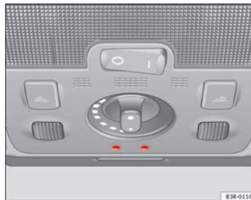
Fig. 92 Detail of headliner: ambient lighting
