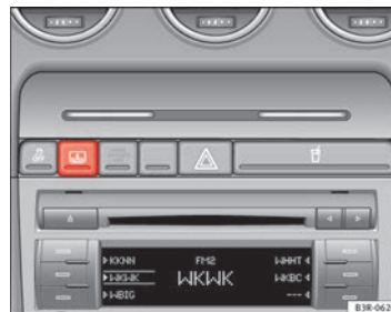
Fig. 98 Switch for electric sun blind on rear window
