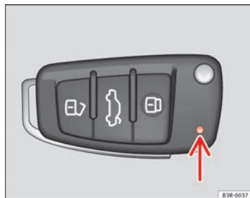
Fig. 68 LED on the remote control key
