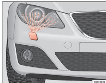
Fig. 100 Headlight with extended washer jet
