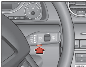
Fig. 61 Windscreen wiper lever: Menu selection button
