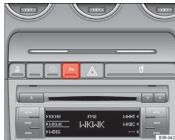
Fig. 142 Centre console: switch for parking aid
