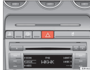
Fig. 89 Centre console: Switch for hazard warning lights
