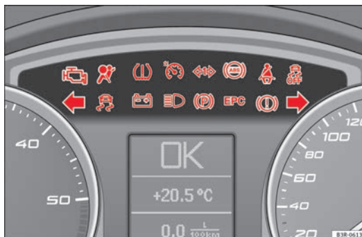
Fig. 44 Instrument panel with warning and indicator lamps
