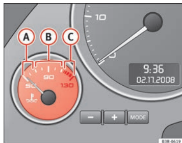
Fig. 38 Engine coolant temperature gauge
