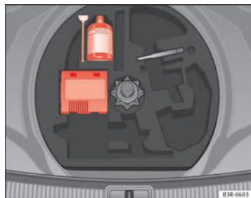
Fig. 180 Tyre Mobility System under floor panel in luggage compartment
