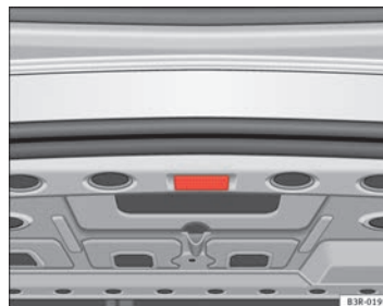
Fig. 94 Detailed view of the top of the luggage compartment: luggage compartment lighting
