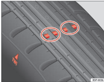
Fig. 177 Tyre tread wear indicators
