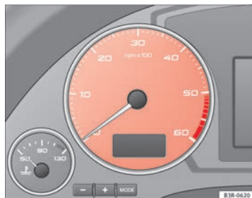
Fig. 39 Detailed view of the instrument panel: Rev counter
