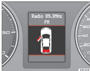
Fig. 51 Display: Door and rear lid warning
