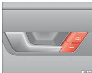
Fig. 71 Detail of the driver door: Central locking switch
