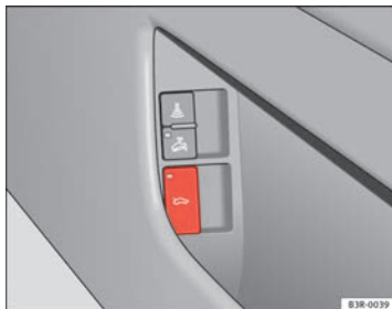
Fig. 74 Driver door: Unlocking the rear lid
