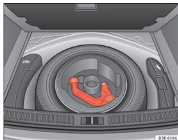
Fig. 154 Luggage compartment: Spare wheel with towing bracket
