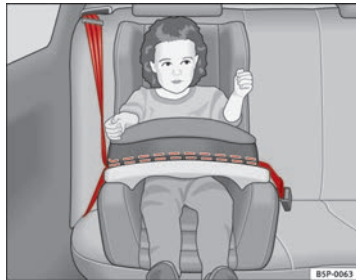
Fig. 30 A category 1 forward-facing child seat fitted on the rear seat.
